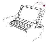
Fold down the touch panel by pressing down on the left and right and on the left and right sides of the panel.
